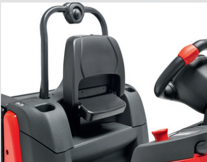
Height adjustable backrest with foldable seating support
