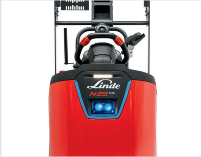
Linde BlueSpot™ and front LED light
