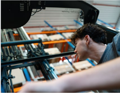
Armoured glass roof for optimal visibility
