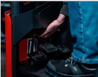
Height-adjustable pedal plate for maximum comfort
